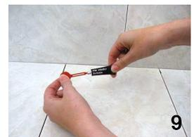
9. Slide the slotted portion of the red tube key over tube end and engage folded end of tube. It may be easier to slightly unfold the tube end before inserting into the red tube key (see pic. 10). Be careful not to squeeze or advance the glue from tube before next step.
