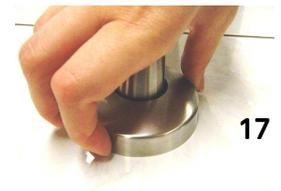
14. Test for proper installation to be sure bar is firmly mounted by applying some pressure.
