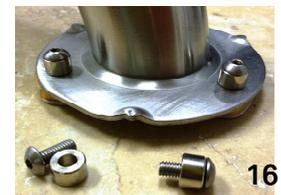
13. Slide cover ring over mounting flange after having ensured tightness of all screws. Turn in one direction until the ring is properly aligned and assure a snug fit. Note there should be a small gap between cover ring and wall to provide proper drainage of water. Pointer: the plate is easily attached if it is turned to the proper position and then snapped on. The ring is concentric and works best when "dialed in place"(see pic. 17).
